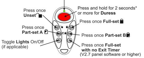
\*This time is programmable - ask your installers for details Normally the RF-Keyfob works in "Quick Key" mode. However, you may ask your installer to set it up for "Secure Unset" mode.
