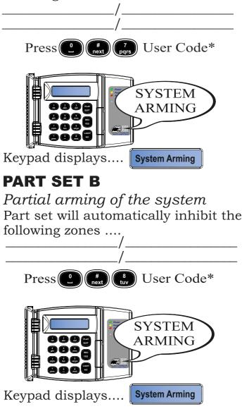
**NOTES:** Zones inhibited in Part Set will remain inactive for the duration of system set.
